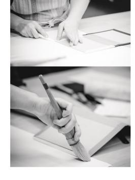
Covering is the process of sticking paper onto a bookbinding board. The bookbinding board and paper must have the same grain direction. The paper is coated with a glue brush and a mixture of bookbinding glue and paste (see explanation of glue types).
